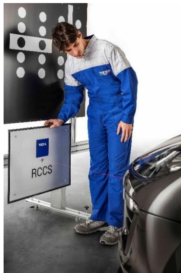
Figure 12: Front radar calibration by using laser technology [20]
