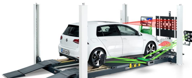
Figure 11: ADAS sensor calibration at the Bosch Workshop [19]
