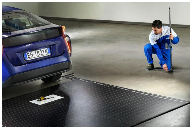
Figure 13: Rear radar calibration by using corner reflector [20]
