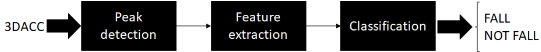
Figure 2: Block diagram of the base line method. Samples are continuously monitored to detect peaks. When a peak is detected, a feature extraction stage takes place. Finally, the extracted features are classified.
