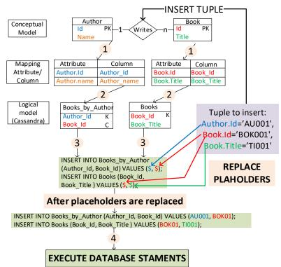
Figure 5 Process of ensuring the logical integrity of data given an insertion of a relationship Writes between a book and an author
