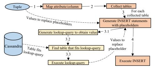
Figure 3 Process of the method to maintain data integrity
