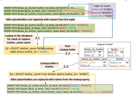
Figure 7 Process of querying information required to maintain the logical integrity
