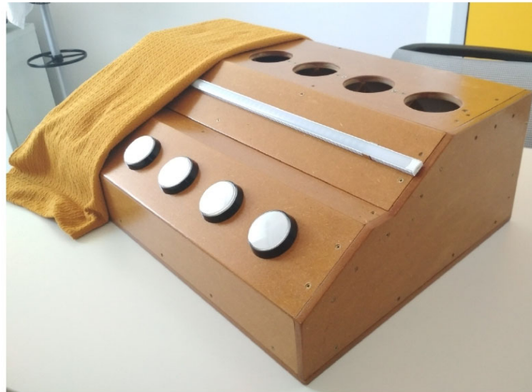
Figure 1. Front view of the Baby-Mnemo device. Four push buttons are available with their 4 corresponding platforms. A blanket is employed to partially cover the device
