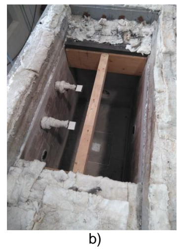
Fig. 1. a) Dimensions of the specimen in mm. b) Specimen assembly inside the furnace.
