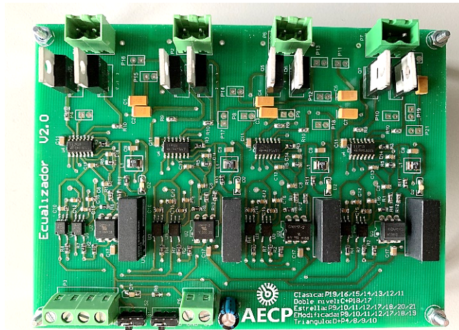
Figure 4.7: SCE prototype for balancing up to 4 cells.
