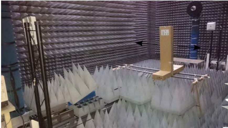
Figure 9: Measurement setup in the anechoic chamber.
