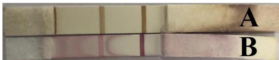
Fig. 5 LFIAs run with red wine samples using (A) superparamagnetic nanoparticles and (B) colloidal gold as reporters
