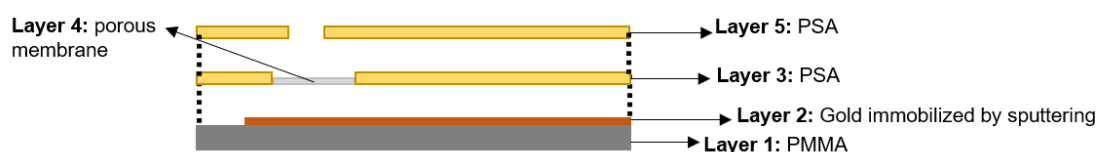
Figure 2. Schematic representation of different layers employed to manufacture the working electrode.
