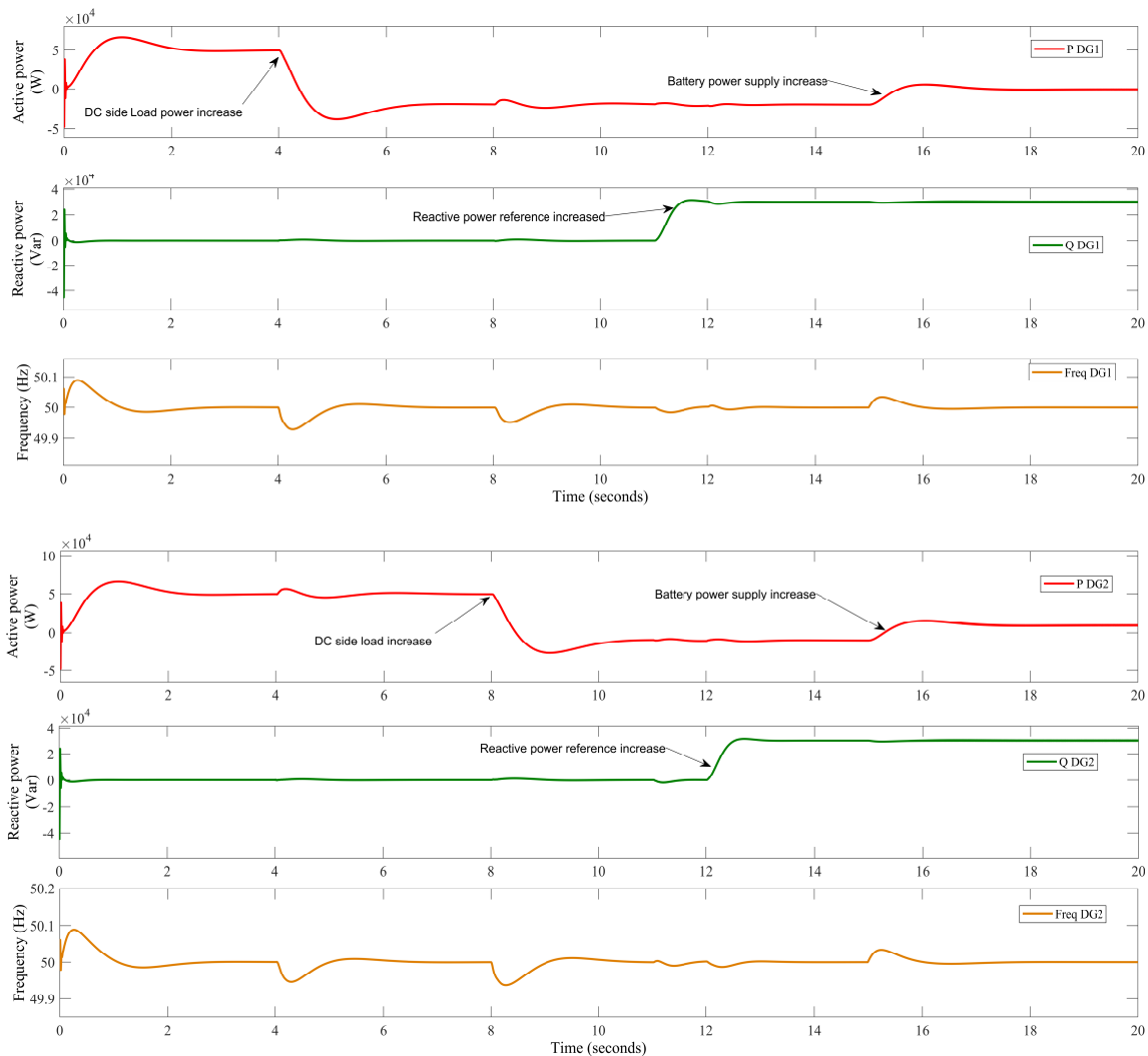
Figure 5-10: Power and frequency simulation results parallel grid connected DC MG( P_{loadDG1} set to 70 kW at 4 s and P_{loadDG2} at 8 s, Q_{refDG1} = 30 kVar at 11 s, Q_{refDG2} = 30 kVar at 12 s and battery supply increase at 15 s)
