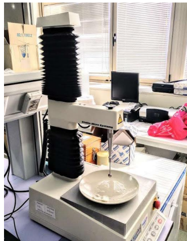
Figura 8. Texturómetro TA.TX plus (Stable Micro Systems)
