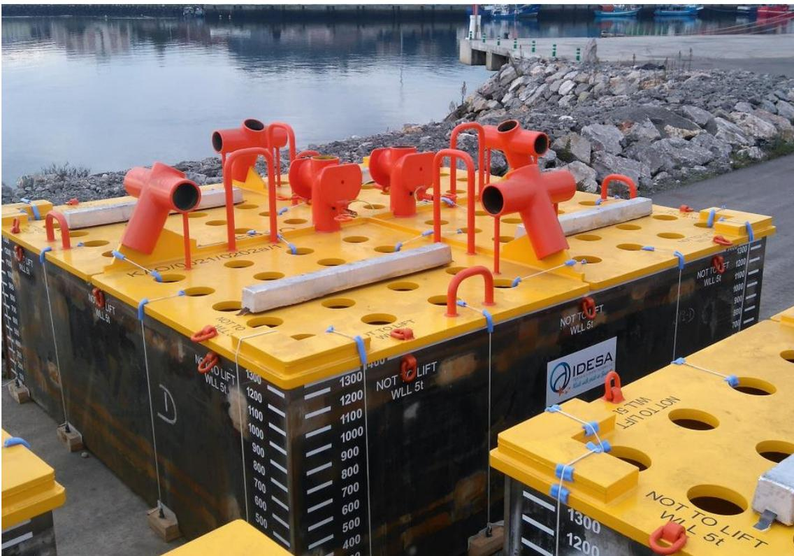
Figura 8: Gravity Bases for Umbilicals [11].
