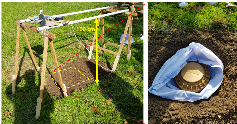
Figure 12. Picture of a 2D-measurement setup (acquisition along x axis). A picture of the anti-tank plastic landmine can be seen in the right picture.
