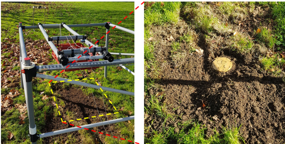
Figure 10. Picture of the measurement setup with an anti-tank plastic landmine buried on the ground. A picture of the anti-tank landmine before burying it can be observed in the right picture.
