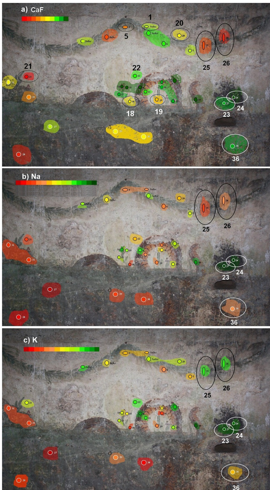
Fig. 1. Qualitative LIBS distribution images of A) CaF, B) Na, C) K in the basement of the House of Ariadne. Red areas correspond to the points with higher relative net intensities, while green areas correspond to lower relative net intensities. (For interpretation of the references to color in this figure legend, the reader is referred to the Web version of this article.)
