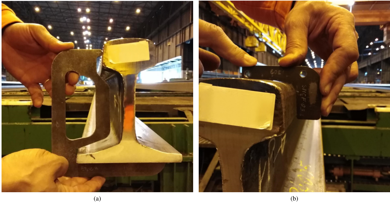
Fig. 2. Positioning the gauge on the rail for manual quality control of the asymmetry after manufacturing.
