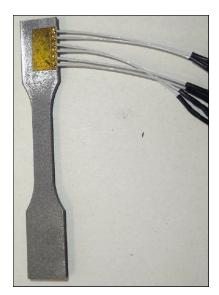
Figure 2. Strain gage method in hole drilling for measurement of residual stresses.
