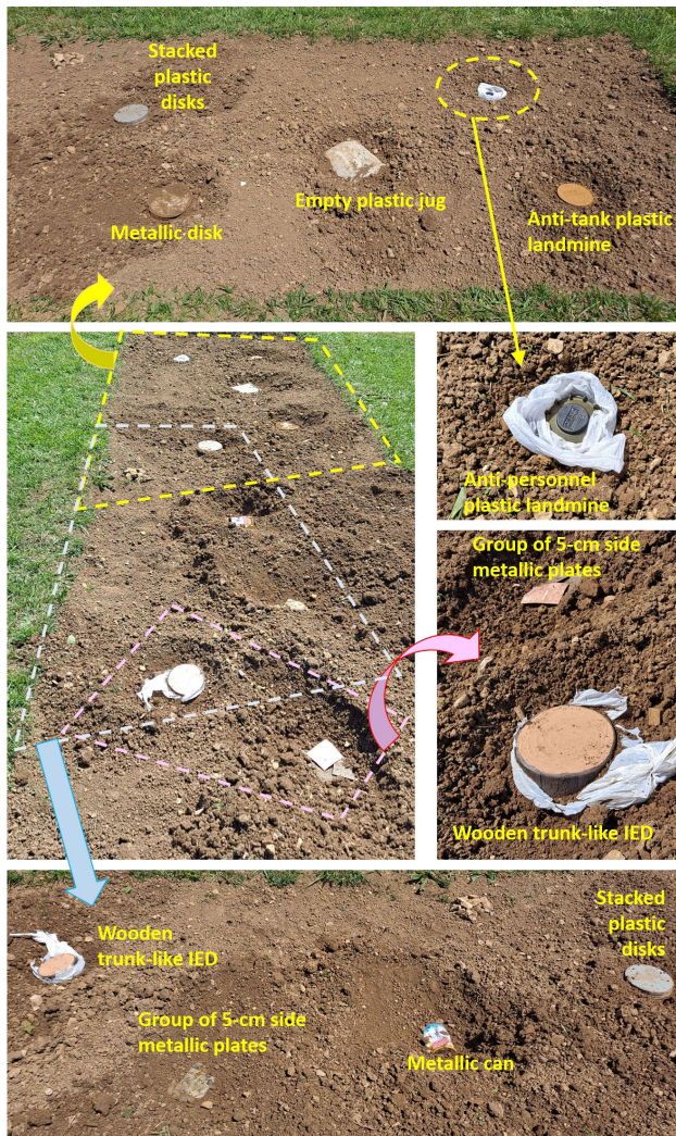
FIGURE 10. Picture of the targets buried in the scanned scenario.
