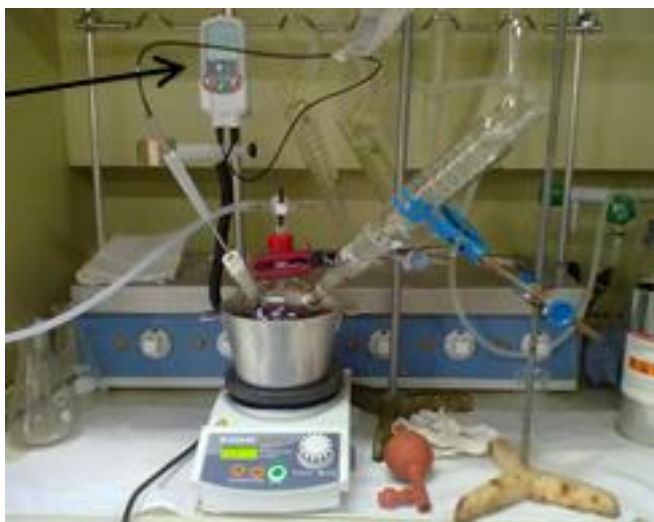
Fig. 11. Synthesis of epoxy-derived samples ( \text{Fe}_3\text{O}_4/\text{GTMO} ).
