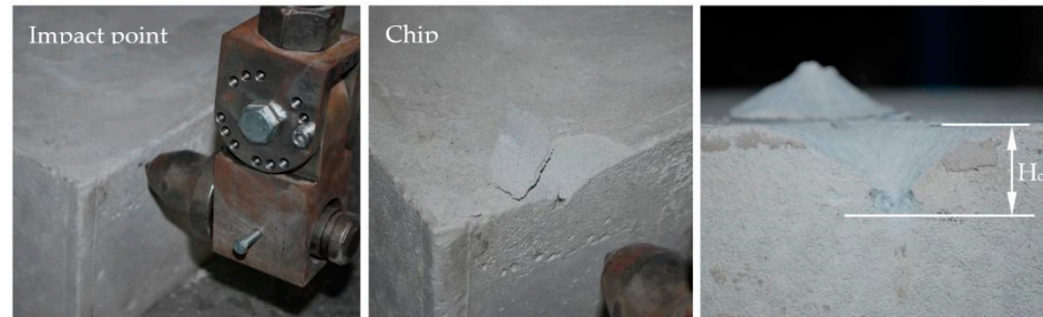
Figure 3. Calculation of the cutting depth as a function of the impact point of the pick on the material.
