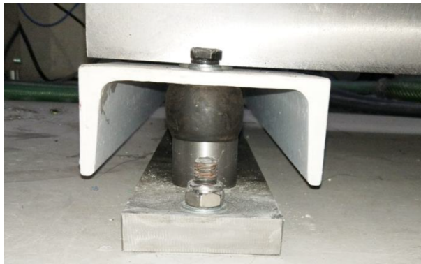
Figure A.4: Test bench attachment to the floor and a rubber shock absorber.
