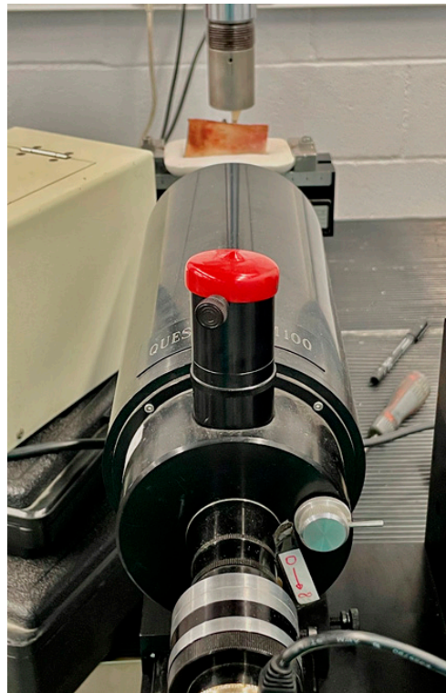
Figure 4. Questar QM-100 long-distance microscope focused on one of the implants in the sample. In the background you can see a rib mounted on its plaster base and mechanized on the base of the load creep machine.
