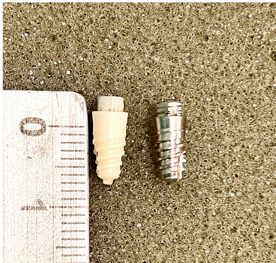
Figure 1. Klockner External Hex SK2 implants, Zr and Ti, both with 3.8*8 buffed surface (Soadco S.L., Escaldes Engordany, Andorra).
