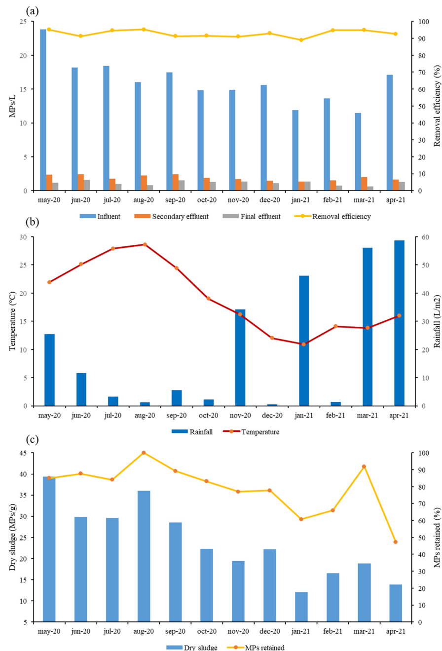
Figure 2. (a) Microplastic concentration (MPs/L) in the WWTP at the four sampling points and overall removal efficiency for one year (May 2020–April 2021), (b) rainfall (L/m 2 ) and temperature (°C) recorded in Caravaca de la Cruz over the sampling period (Source: State Meteorological Agency [38]), (c) Microplastic concentration in sludge expressed per dry weight (MPs/g) and percentages of MPs retained in the sludge with respect to the MPs removed during the treatment in the WWTP during the period studied.
