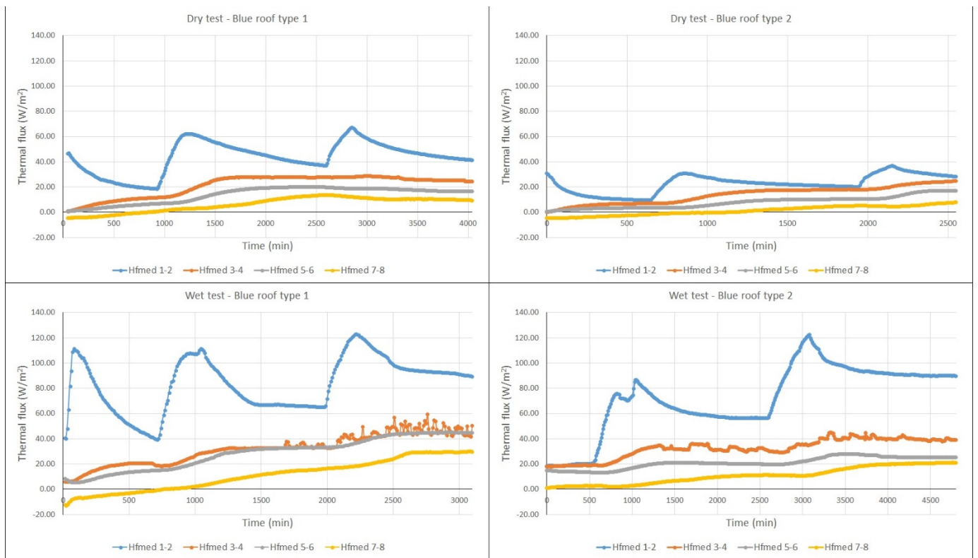
Figure 4. Heat flux in types 1 and 2 of the blue roofs under dry and wet conditions.
