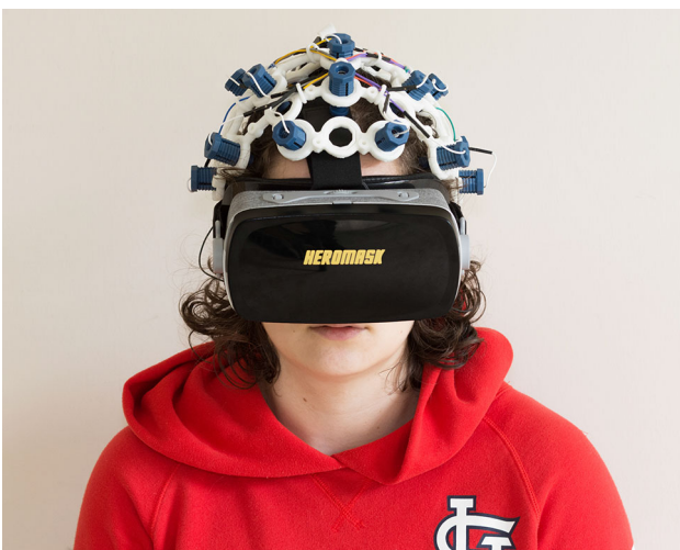
Fig. 2 VR-Photosense set-up with a cardboard viewer and an OpenBCI EEG headset
