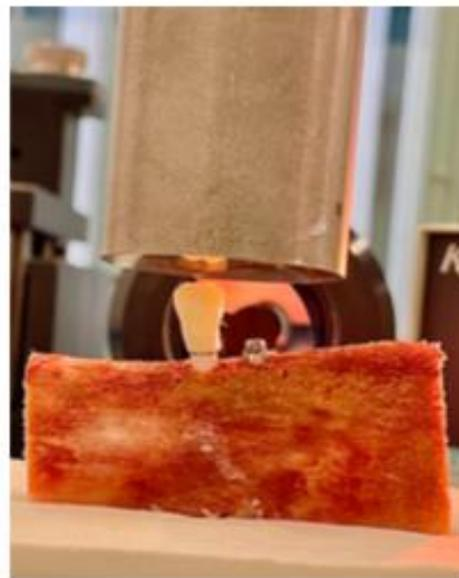
**Figure 5.** Detail of the PMMA crown screwed on the external hexagon of the Zr implant, and mounting on the MTS Bionix 358 test machine. In the background you can see the lens of the Questar QM-100 long-distance microscope.
