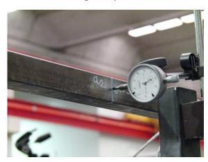
Figure 8. Mounting of the dial gauge for the displacement measurement of the a2 section.
