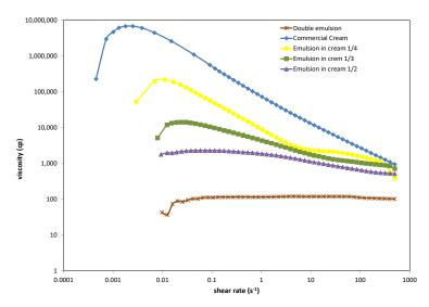
**Figure 4.** Viscosity measurements of the commercial cream and mixtures of the commercial cream with the double emulsion  $W_1/O/W_2$  of concentration 80/20 with an internal phase ratio  $W_1/O$  of 30/70.
