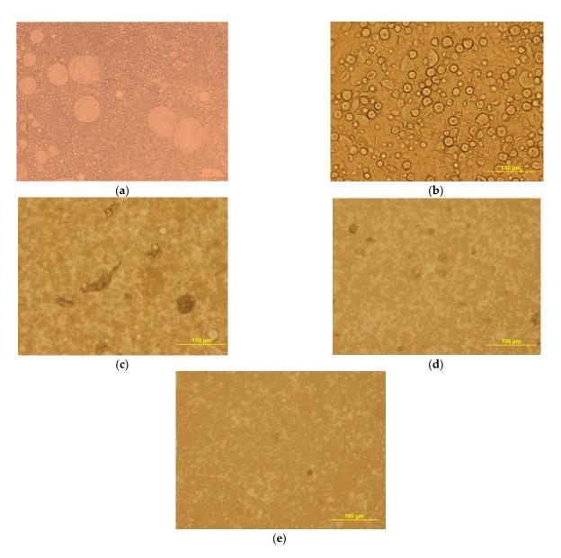
**Figure 2.** Micrographs of the commercial cream and mixtures of the commercial cream with the double emulsion  $W_1/O/W_2$  of concentration 80/20 with an internal phase ratio  $W_1/O$  of 30/70: (a) double emulsion; (b) commercial cream; (c) commercial cream with 1/4 emulsion; (d) commercial cream with 1/3 emulsion and (e) commercial cream with 1/2 emulsion.
