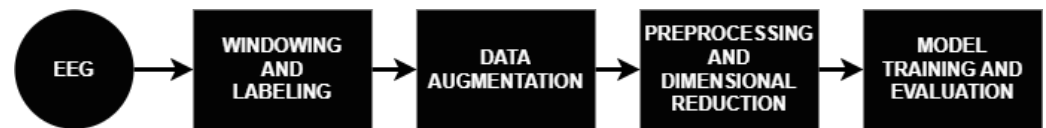
Figure 3. Workflow of this research. The original EEG data from the dataset are windowed and labeled. The Cross-Validation introduces a subsampling for reducing the number of non-PPR windows, while DA takes place to balance the number of PPR windows in the training/testing dataset. Window preprocessing, feature extraction, and dimensional reduction are applied to each EEG window. Finally, the process ends with the training and testing of the models.
