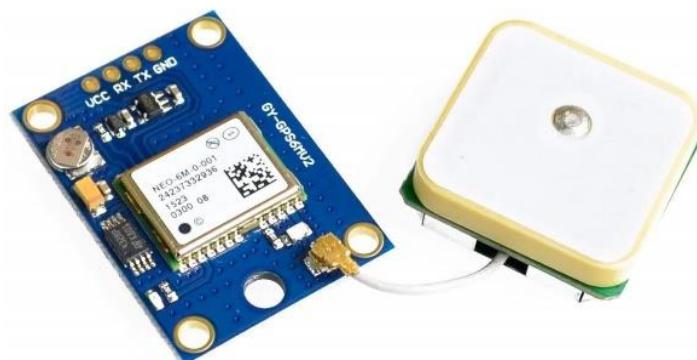
Figure 31 - The GPS module Neo-6M
