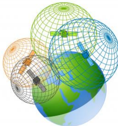
Figure 9 - Trilateration of 4 satellites
