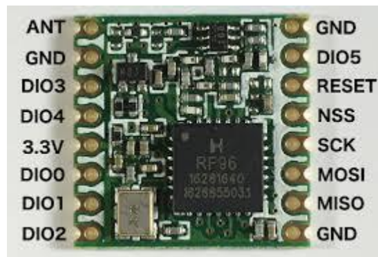
Figure 33 - The LoRa module RFM95 (not used in the end)
