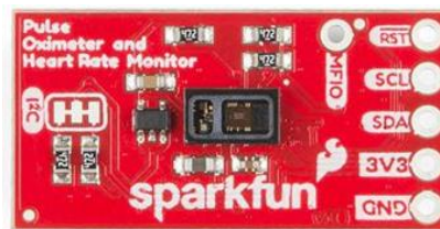
Figure 13 - Single-part pulsimeter device (19)
