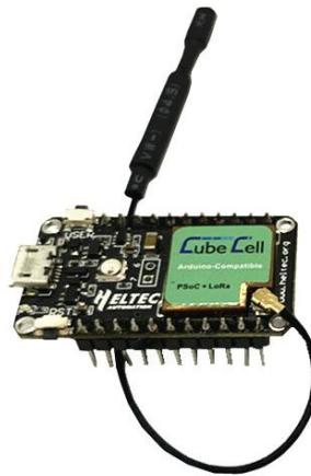
Figure 20 - Heltec Cubecell HTCC-AB01, including the LoRaWAN antenna
