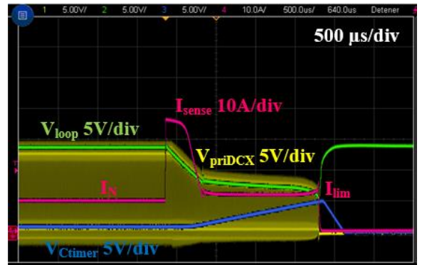
Fig. 11. Class 10 LCL operation waveforms using the SCT3022AL SiC N-MOS
