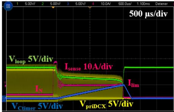
Fig. 14. LCL operation under overload test using and LC filter between the LCL and the load using the SCT3022AL SiC N-MOS
