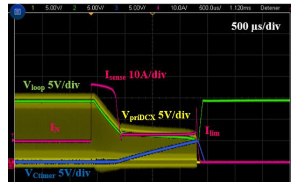
Fig. 12. Class 10 LCL operation waveforms using the SCTW90N65G2V SiC N-MOS
