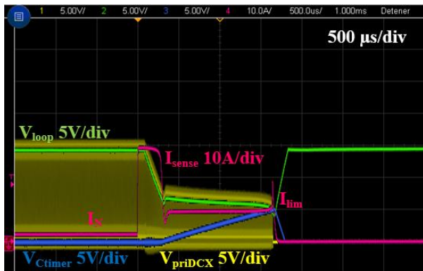
Fig. 15. LCL operation under overload test using and LC filter between the LCL and the load using the SCTW90N65G2V SiC N-MOS
