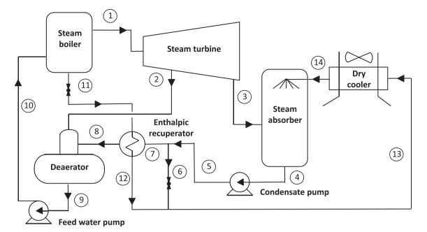
Fig. 1. Scheme of the Hygroscopic Cycle Technology.
