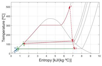
Fig. 10. T-s diagram of RC.
