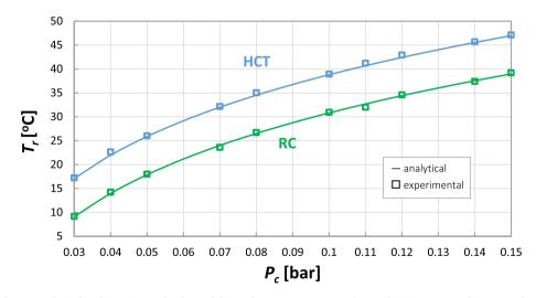
Fig. 6. Analytical and experimental values of the cooling temperature vs. the condensing pressure for HCT and RC.
