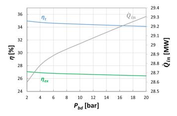
Fig. 20. Thermal and exergy efficiencies and thermal power input vs bleeding pressure.
