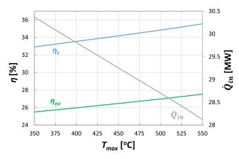
Fig. 22. Thermal and exergy efficiencies and thermal power input vs maximun temperature of the working fluid.
