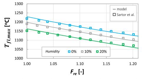
Fig. 8. Comparison between the values obtained with the model of the boiler and the values obtained by [42] for the maximum flame temperature vs. relative air-fuel ratio with different humidity percentages of the biomass presented in [42].
