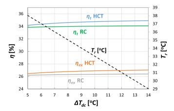
Fig. 18. Thermal and exergy efficiency vs. temperature difference of the working fluid in the dry coolers for HCT and RC.
