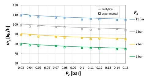
Fig. 4. Analytical and experimental values of the mass flow rate vs. the condensing pressure for different pressures in the boiler.
