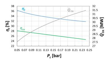
Fig. 19. Thermal and exergy efficiencies and thermal power input vs condensing pressure.
