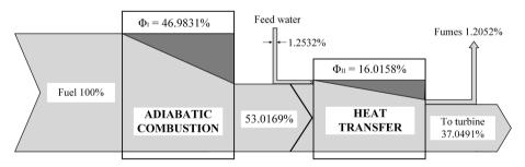
Fig. 13. Grassmann diagram of the RC boiler.
