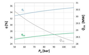
Fig. 21. Thermal and exergy efficiencies and thermal power input vs boiler pressure.
