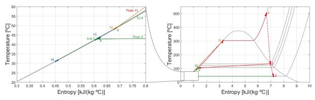
Fig. 9. T-s diagram of HCT.
