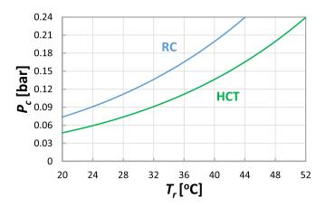
Fig. 15. Condensing pressure vs. cooling temperature for HCT and RC.
