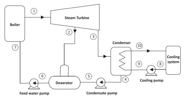
Fig. 2. Scheme of the regenerative Rankine Cycle with deaerator.
