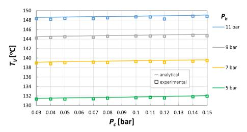
Fig. 5. Analytical and experimental values of the temperature of the vapor at the inlet of the condenser/absorber vs. the condensing pressure for different pressures in the boiler.
