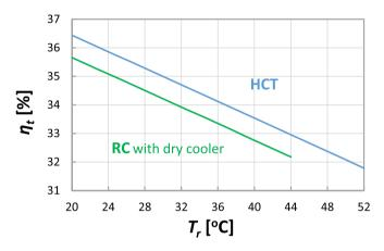
Fig. 16. Thermal efficiency vs. condensing temperature for HCT and RC with dry cooler.
