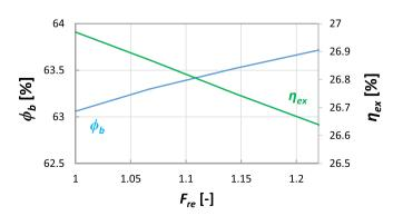
**Fig. 23.** Exergy destruction ratio in the boiler and exergy efficiency of the HCT vs relative air–fuel ratio.
