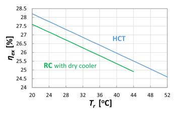
Fig. 17. Exergy efficiency vs. cooling temperature for HCT and RC.
