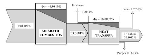
Fig. 14. Grassmann diagram of the HCT boiler.
