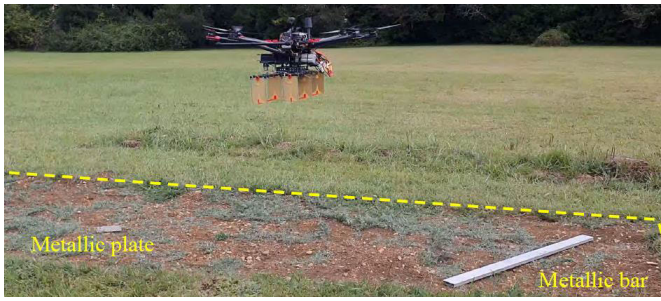
Fig. 10. Picture of the array-based GPR-SAR system on board the UAV.
