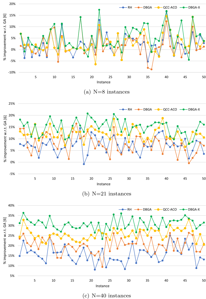
Fig. 11. Comparison of DBGA-X with previous state of the art methods RH [11], DBGA [3] and QCC-ACO [12]: percentage improvement in makespan with respect to GA [10] in all 50 instances of each of the (a) N = 8 , (b) N = 21 and (c) N = 40 benchmarks.
