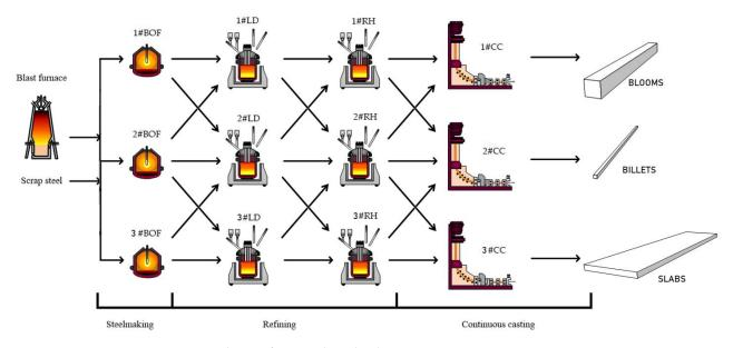
Figure 1. Phases of a typical Steelmaking Continuous Casting process.
