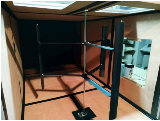
Fig. 2. Three-bladed H-VAWT installed inside an hybrid modular enclosure for the test chamber of the XAWT wind tunnel.
