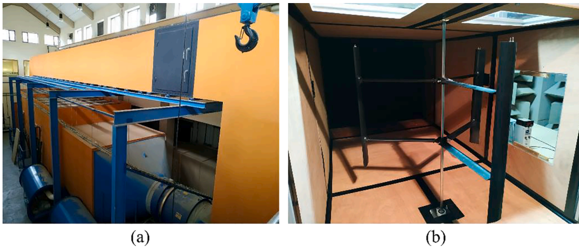
Fig. 1. a) Picture of general overview of the wind tunnel. b) Turbine prototype inside the test section of the wind tunnel.
