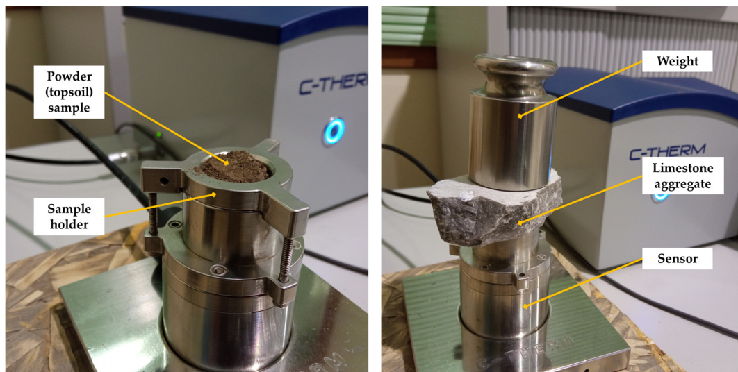
Figure 2. Measurement of thermal conductivity with C-Therm ® TCI analyzer: powder test (left) and solid test (right).
