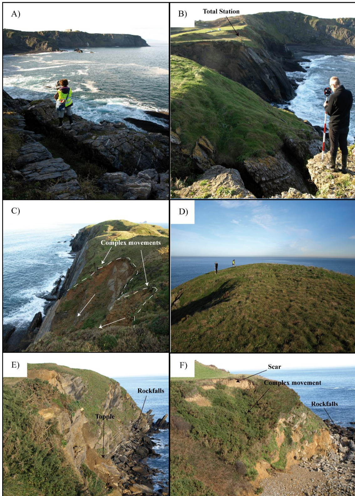
Figure 91. A) and B) Topographic monitoring field campaign by means of total station in western side of Podes. C) Several complex gravity movements observed at the cliff edge. D) Location where PS with VLOS 12.9 \text{ mm year}^{-1} were detected. E) and F) Coastal instabilities developed on the east side of Podes. Photos taken in January, 19 2021. Taken and modified from Cuervas-Mons et al. (2021b) .
