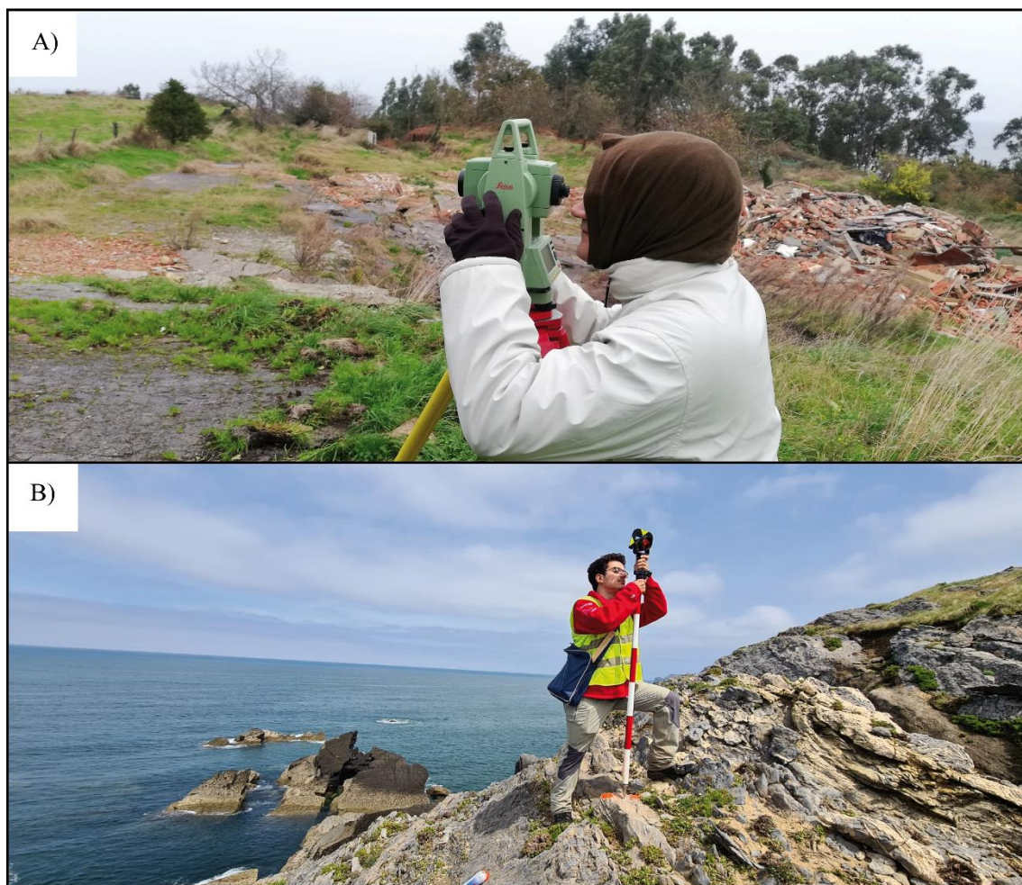
Figure 82. Topographic monitoring field campaign by means of total station in A) Tazones Lighthouse landslide and B) Podes Peninsula.
