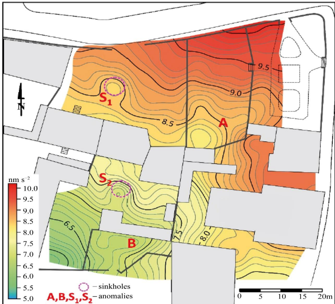
Figure 24. Gravity method applied to subsidence related to underground mining activities: Distribution of anomalies of gravity (Bouguer anomalies) and distribution of buildings, mining facilities and sinkholes. Taken and modified from Porzucek and Loj (2021) .
