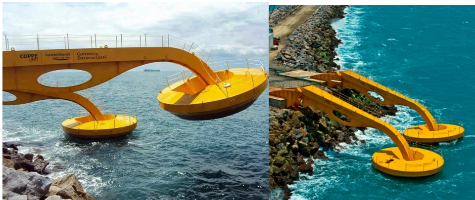
Fig. 2.6: Seahorse power take-off system
