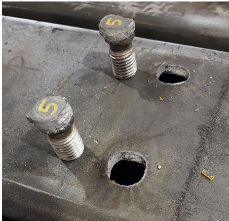
Figure 3 Failure mode of SCS5 specimen.
