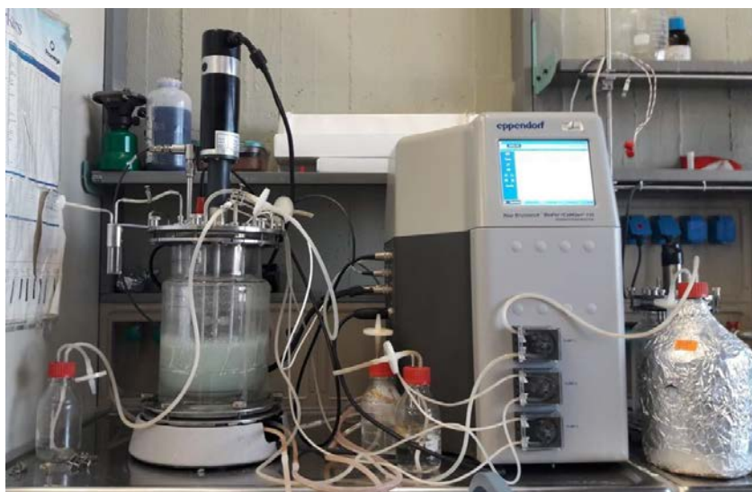
Figure 2.1. POXA1b production from P. pastoris in 5 L-scale fermenter.
