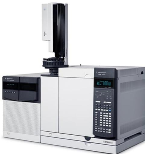
**Figura 28.** GC-EI-MS/MS Agilent 7000C.
